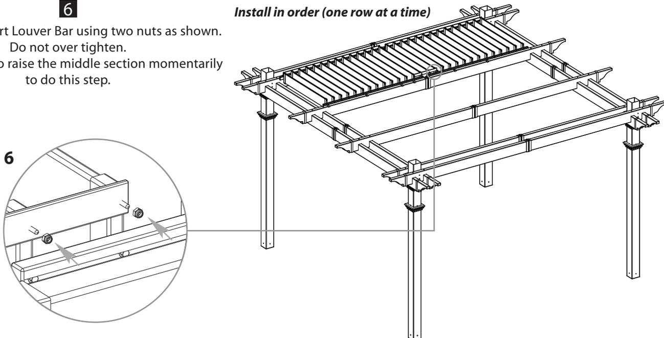
**Note:** check that the holes are closer to the bottom as shown.
