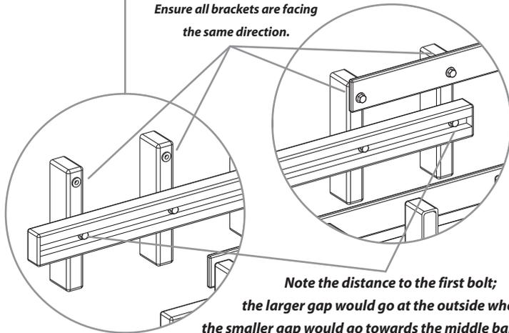
**Note the distance to the first bolt; the larger gap would go at the outside whereas the smaller gap would go towards the middle bar assembly.**
