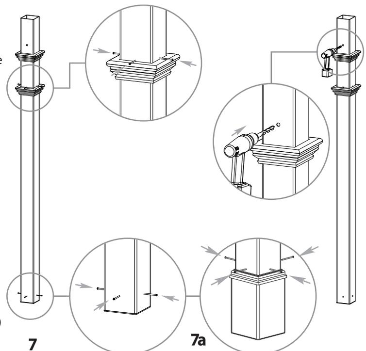
At this stage, the columns should be properly installed as per the following illustration, with the columns 134" in. (340.4 cm) apart. Also, notice that the holes at the top of each post should be facing the same direction.
