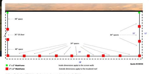
Walls are 8' tall with an 18" kickplate. Single outswing door quoted. Insulated roof is 4" thick
