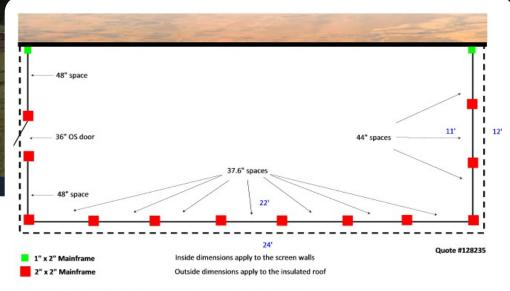
Walls are 8' tall with an 18" kickplate. Single outswing door quoted. Insulated roof is 4" thick
