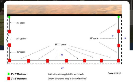
Walls are 8' tall with an 18" kickplate. Single outswing door quoted. Insulated roof is 3" thick
