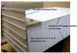
Hereiner betreasten Facinge: 024: alursisem alkay Facinge: 024: alkay Facinge: 024: alursisem alkay Facinge: 024: alkay Facinge: This above is a cutaway of the roof section. It is available in 3", 4" & 6" thicknesses all with the specially formulated polystyrene core with an .024 laminated aluminum skin on both sides. Shown here with the extruded aluminum fascia screwed into place.
