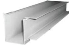
**TIP:** When installing the gutter over the panels, be sure the panels sit square inside the channel. If not installed properly, the gutter will install at an angle and will not be capped properly by the side fascia.
